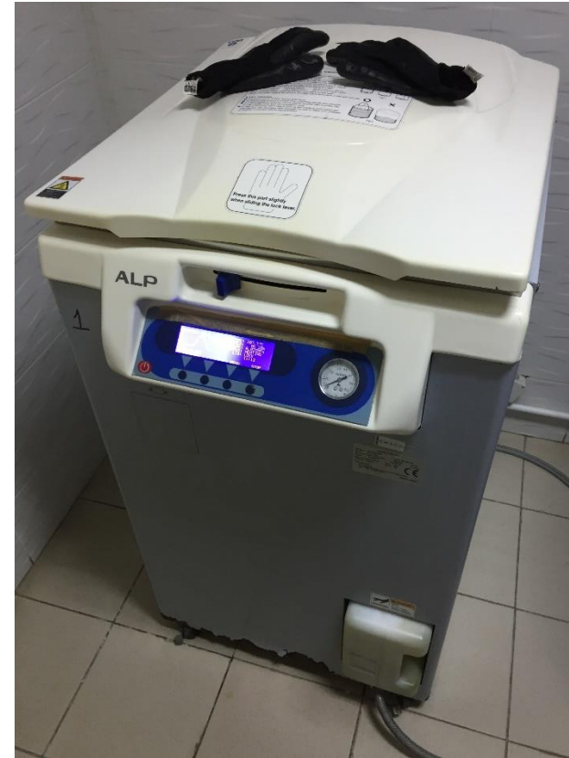
Right: autoclave in use for biological waste management in medical facility
